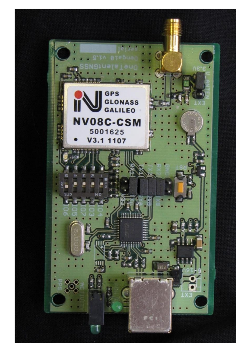
Fig. 2: Denga10 GNSS receiver with GNSS-Chip from NVS
